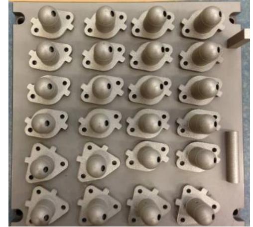
Example of the manufacturing plate for Injectors. The position of parts is frozen
