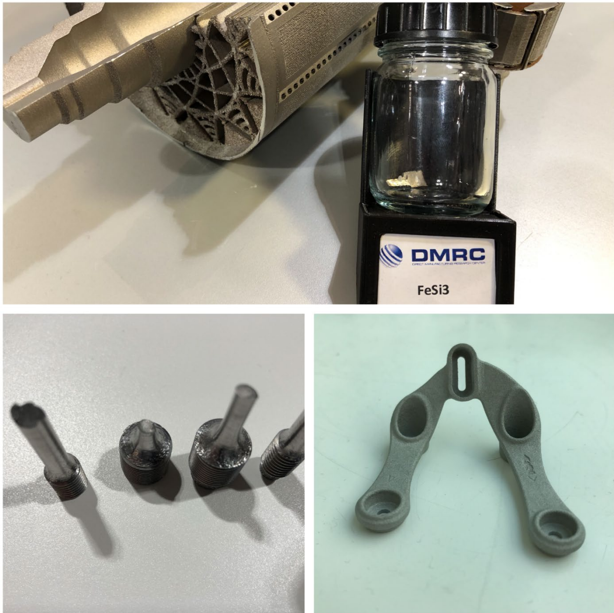
Figure 6 Novel electric motor designs and new materials from DMRC, the ambitious AMCOCS (Additive Manufactured Component Certification Services) and serial production binder jet parts in Ti6-4 from Fraunhofer IFAM
